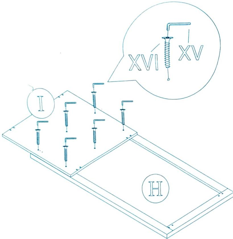
Join panel [I] to panel [H] by screw in 6x screws (XVI) into corresponding holes and tighten with allen key (XV).
