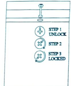
*PLEASE PUSH THE DRAWER SLIDES UNTIL THE END ACCORDING TO THE ARROW'S DIRECTION SHOWN ABOVE.*
