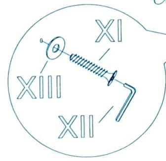
Join metal (VIII)x2 (IX)x2 by using 4x washer (XIII) and 4x screw (XI) and tighten with allen key (XII).
