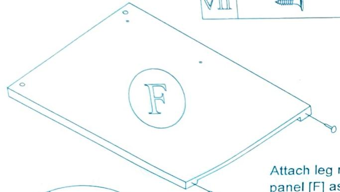
Attach leg nail (V) into panel [F] as shown with a hammer.
