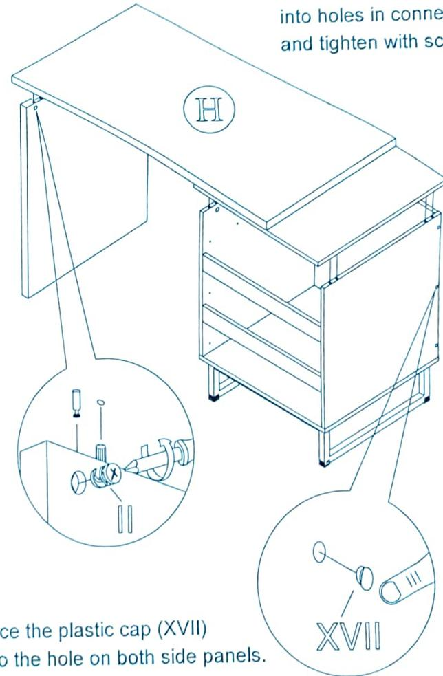
Place the plastic cap (XVII) in to the hole on both side panels.
