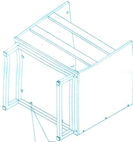
Attach assemble metal to base of panel [E] by using 8x screw (VII). Fasten all screws.
