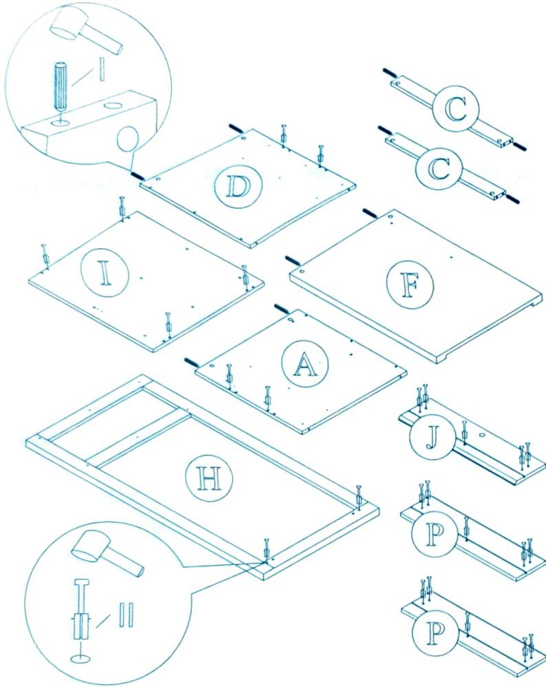
Insert 10x dowel (I) and 25x pin (II-pin) into all panel as shown.
