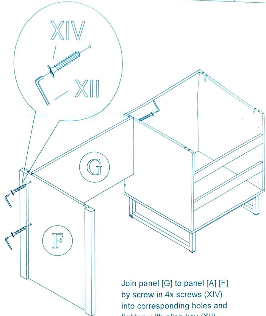
Join panel [G] to panel [A] [F] by screw in 4x screws (XIV) into corresponding holes and tighten with allen key (XII).
