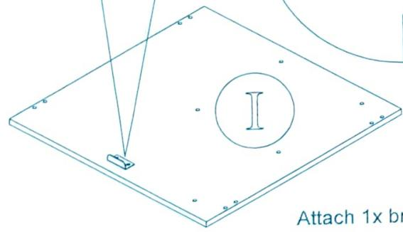
Attach 1x bracket (VI) in panel [I] using 2x screw (VII).
