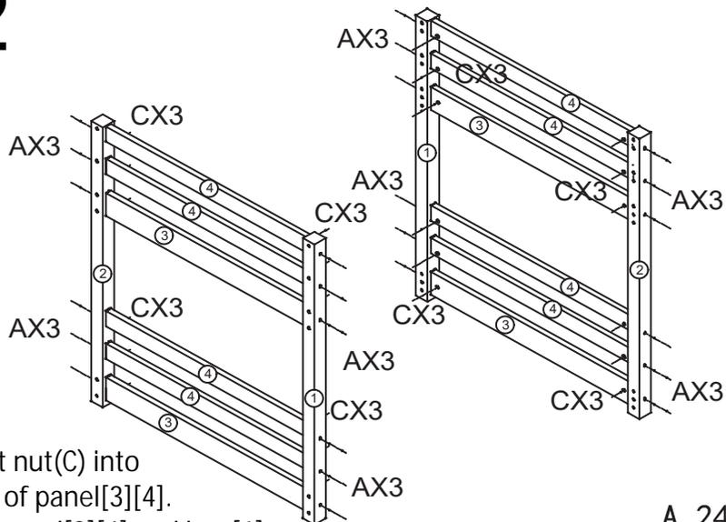
Insert nut(C) into sides of panel[3][4].
