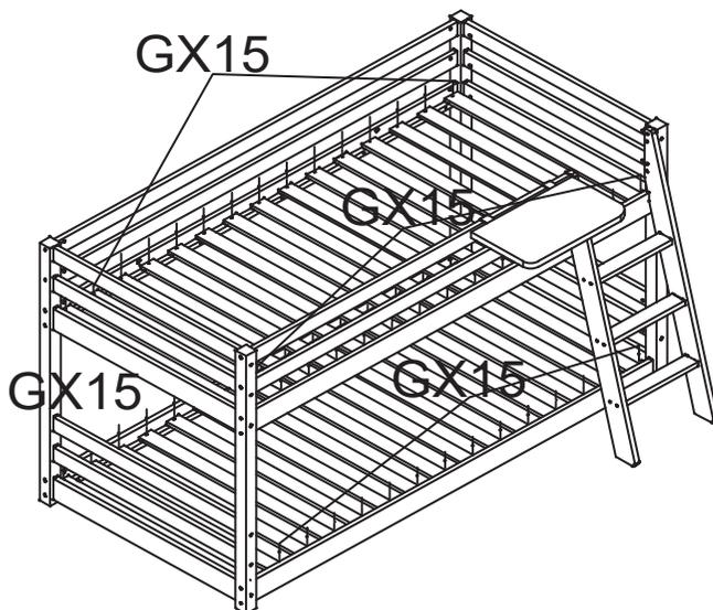
Insert 60x screw(G) into the holes of slats as shown.
