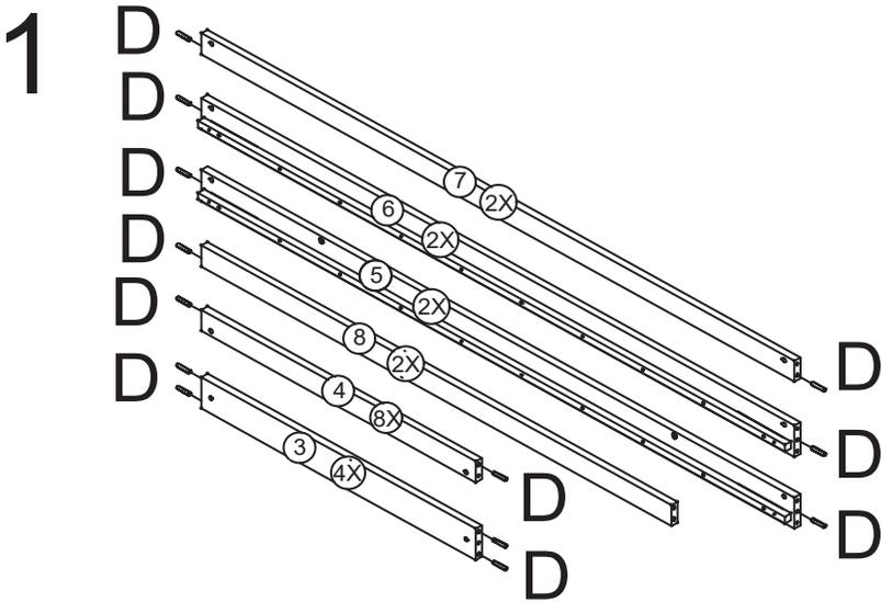
Insert dowel (D) into panel[3][4][5]
